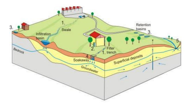
The above diagram shows the flow of water through sustainable drainage systems into the subsurface during a storm event.
